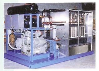
**A&V** Ice Makers produce a hard cracked ice ideal for seafood & poultry, fresh vegetable processing, industrial catering, the chemical & concrete business, plus the wholesale and retail food industries. Thickness of the ice is adjustable from 1/8" to 5/8", allowing for great flexibility.
